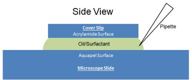
b.) Once the chamber is filled with oil/surfactant, flow in the water very <u>slowly</u> and displace the oil. We often use a Kimwipe at one end of the chamber to wick out the oil while pipetting in the water phase at the other end. You should see an oil/water interface moving across the channel.
