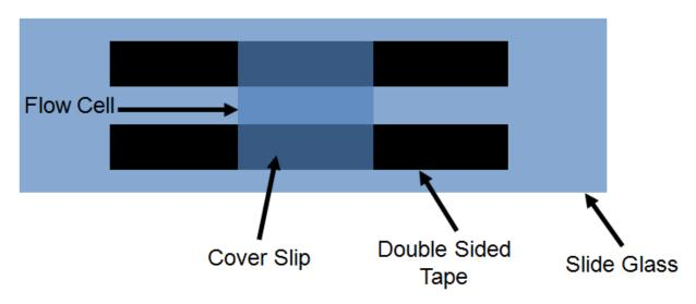
A 100 $\mu$ m thick and ~3mm wide channel will only require ~<u>5 $\mu$ l</u> of volume to fill.
