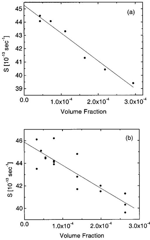
FIG. 4. (a) Concentration-dependent sedimentation velocity  $S'$  [Eq. (C5)] for  $fd$  at 50 mM ionic strength. The data are fitted to a linear function  $S' = 45.3 - 20980\phi$ . The solid line is given by Eq. (C6), which yields  $\alpha S_0$ . The overlap volume fraction for  $fd$  with  $L = 880$  nm is  $5.9 \times 10^{-5}$ . (b) Concentration-dependent sedimentation velocity for  $fd$  at 100 mM ionic strength. The data are fitted to a linear function  $S' = 45.9 - 20450\phi$ .
