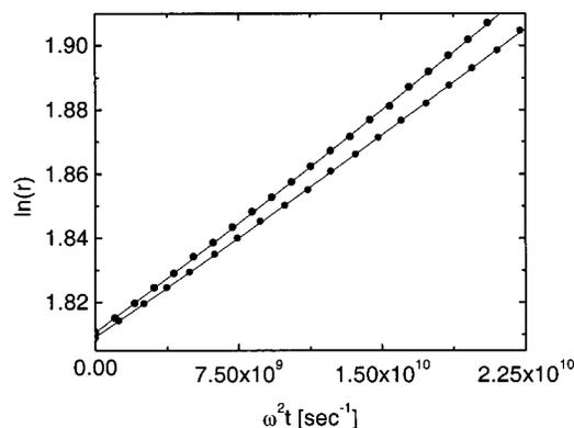
FIG. 7. Position of the sedimentation boundary plotted against  $\omega^2 t$ . The circles represent measurements which were taken approximately every 2.5 min. The lines represent the second-order polynomial fit to the data [Eq. (C2)]. The plot with a larger slope corresponds to the sedimentation of *fd* virus in 100 mM ionic strength at a volume fraction of  $7.75 \times 10^{-5}$  at 25 000 rpm. The other plot is for a higher volume fraction of *fd* equal to  $2.63 \times 10^{-4}$ .
