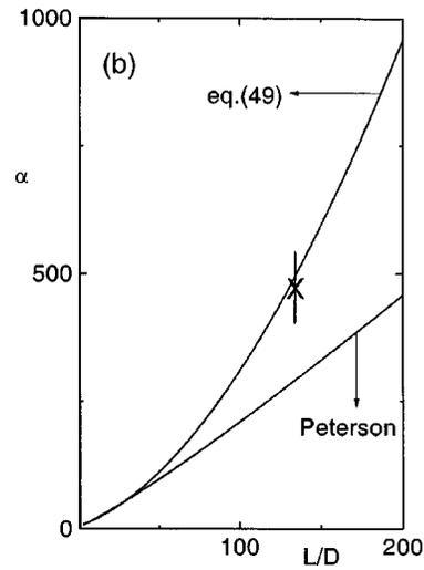
FIG. 1. (a) The dependence of the coefficient  $\alpha$  on  $L/D$  according to Eq. (49) and to Peterson (Ref. 3). The coefficient  $\alpha$  is the first-order correction to the sedimentation velocity due to finite concentration of the colloidal rods. The two data points are for silica rods. (b) The coefficient  $\alpha$  for  $L/D < 200$ . The data point is for the *fd* virus, as obtained in Sec. IV.
